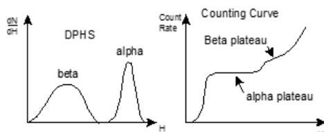
Figure 3: Curves for both alpha and beta particle. LEFT: Differential Pulse Height Spectrum (DHPS) RIGHT: Counting Curve. [2]
