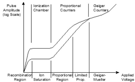
Figure 2: Pulse-height vs Voltage in a gas filled detector [2]
